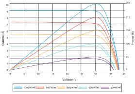
Excellent performance under weak light conditions: at an irradiation intensity of 200 W/m $^2$  (AM 1.5, 25 °C), **96.5**% or higher of the STC efficiency (1000 W/m<sup>2</sup>) is achieved
