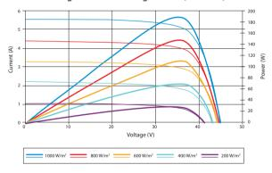
Exellent performance under weak light conditions: at an irradiation intensity of 200 W/m $^2$  (AM 1.5, 25 °C), 95.5% or higher of the STC efficiency (1000 W/m $^2$ ) is achieved
