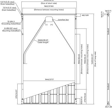
$<sup>\</sup>ensuremath{^{*}}$  The distance between the center of the mounting/grounding holes
